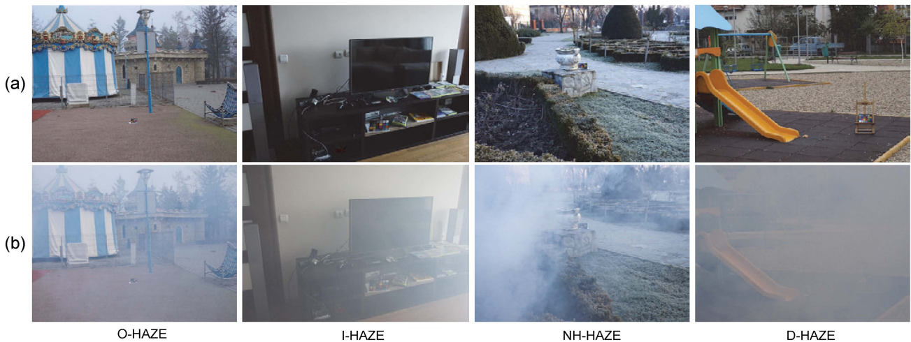
Fig. 3. Example images from O-HAZE [12], I-HAZE [13], Dense-haze [14], and NH-HAZE [15]. (a) is the reference, and (b) is the corresponding hazy images. The hazy images and corresponding references are almost components aligned with spatial and background. However, since the haze is machine-generated, the haze of hazy images looks unnatural and more like smoke.
